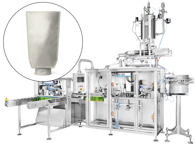
The plastic pouches manipulated in the pilot case and the machinery where they have to be placed for filling
