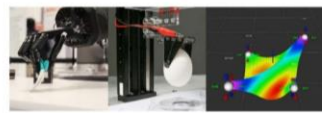
Three initial implementation solutions to be merged into the MERGING platform: (left) Shadow Hand, (center) EPFL's soft gripper based on electro-adhesion, (right) flexible material modeling for robotic handling
