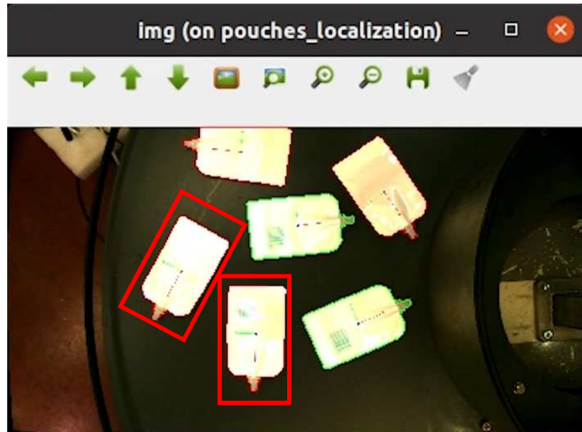
Figure 9 : VISION MODULE: Default with pouches detection: In red the faulty pouches
