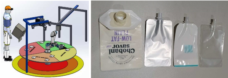
Figure 37. Layout for THIMONNIER use-case 1 (left); pouches to be localized (right).
