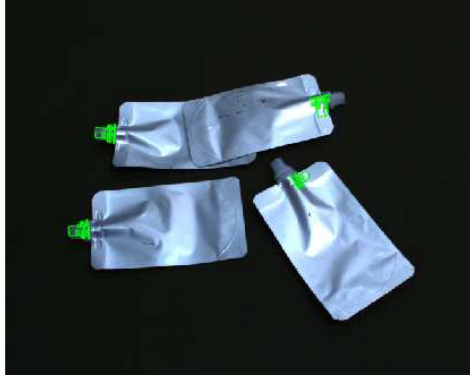
Figure 42. Detection of bottlenecks of grey pouches (detection in green colour).
