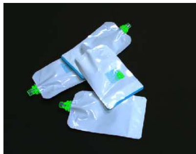
Figure 41. Wrong detection in white pouch (detection in green contour).
