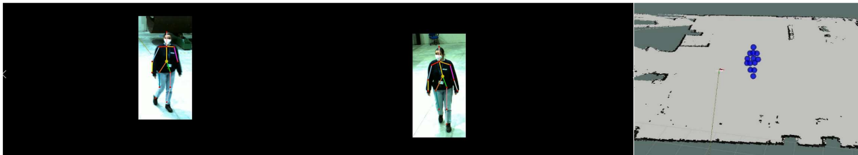
Figure 11. Movement decomposition system output: result of OpenPose in 2D images previously filtered by YOLO neural network (left); Output represented in Rviz in 3D (right).
