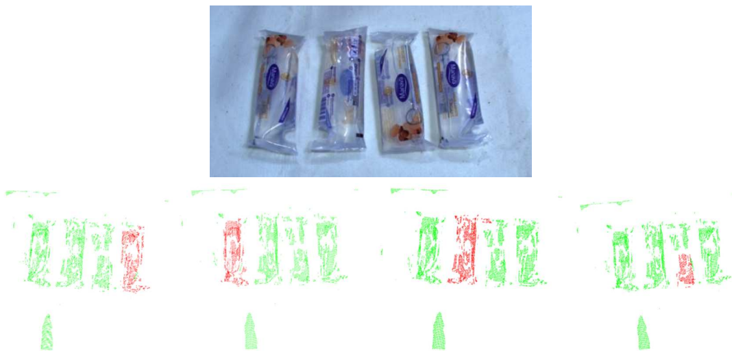
Figure 50. Original 2D capture and cluster extraction for transparent pouches.
