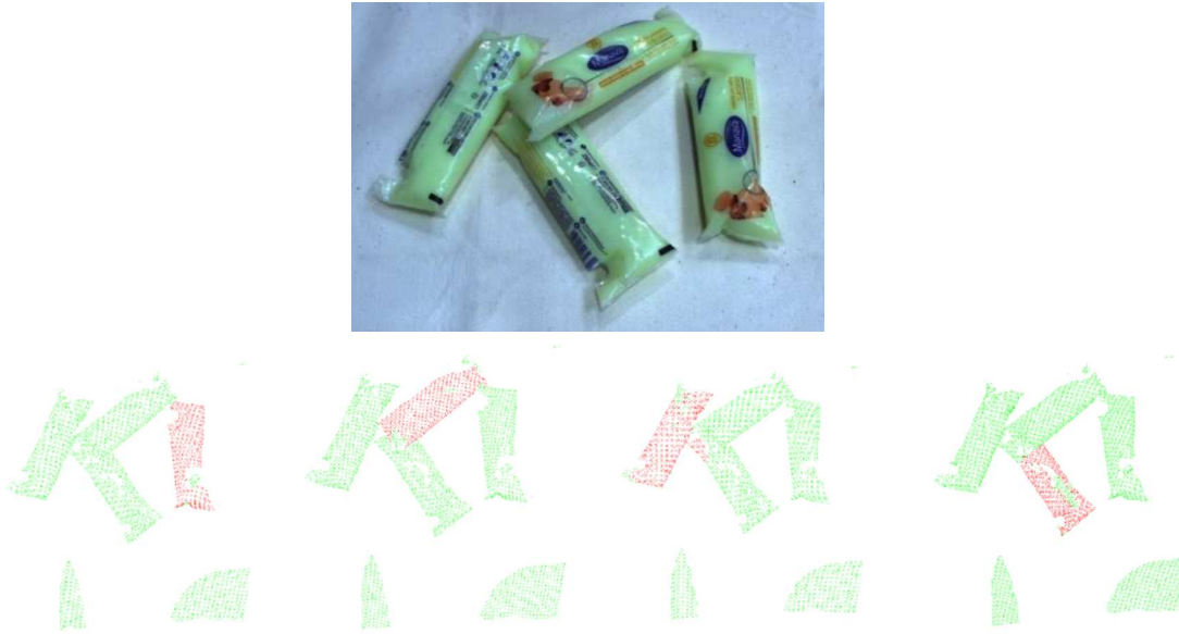
Figure 53. Original 2D capture and cluster extraction of overlapped green pouches.
