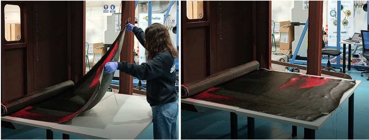
Figure 56. Ply absorbing the projected light in some areas.
