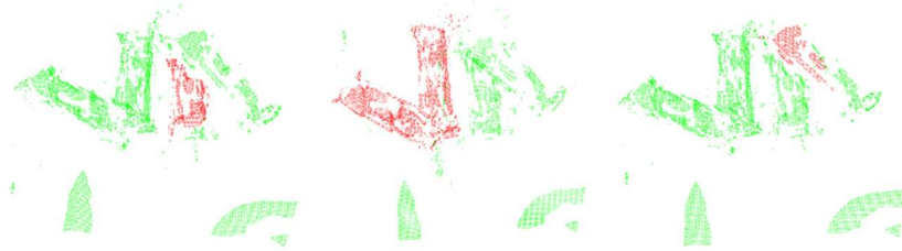
Figure 51. Original 2D capture and cluster extraction for overlapped transparent pouches.
