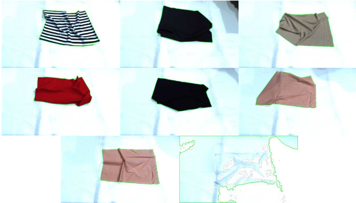
Figure 21. Result of the segmentation algorithm for several types of fabric: the fabric is correctly segmented except for the white one.
