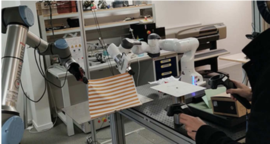
Figure 34 - Selmark experimental setup, using bi-manual MoCap teleoperation for gesture teaching
