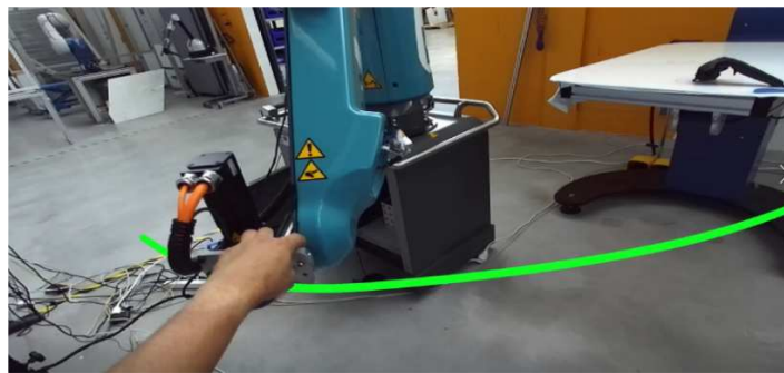
Figure 55. Display of the view of the operator. In green the virtual guide in the real scene
