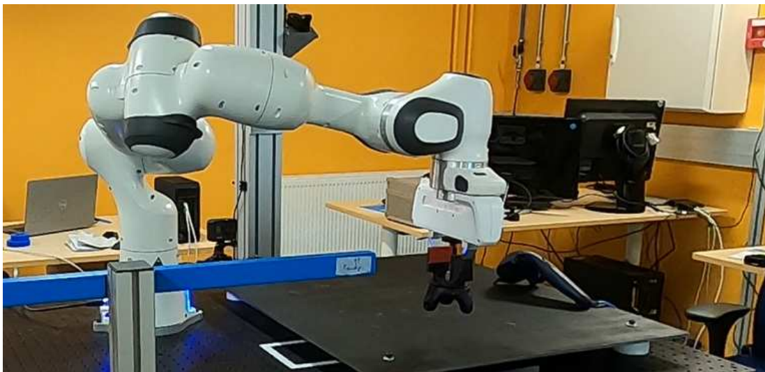
Figure 6 - Calibration with the motion capture tracker fitted on the robot
