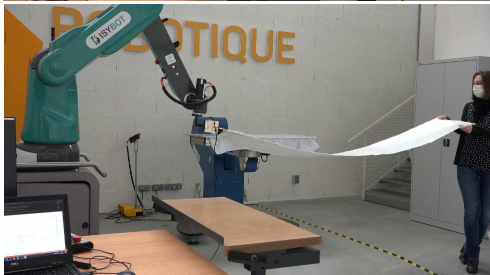
Figure 54. Co-manipulation of flexible objects with different length
