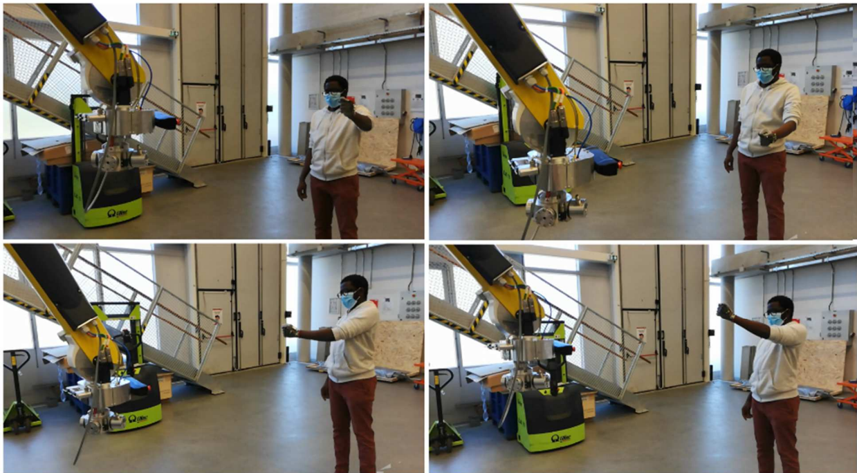
Figure 39 Testing the position control loop
