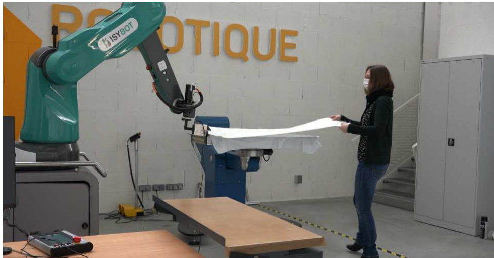
Figure 53. Co-manipulation of objects with different thickness and length
