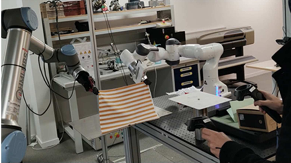
Figure 15 - Bimanual teleoperation for Selmark ply manipulation
