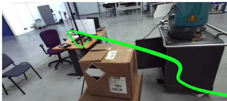
Figure 59. Modified guide that enables to avoid the obstacle
