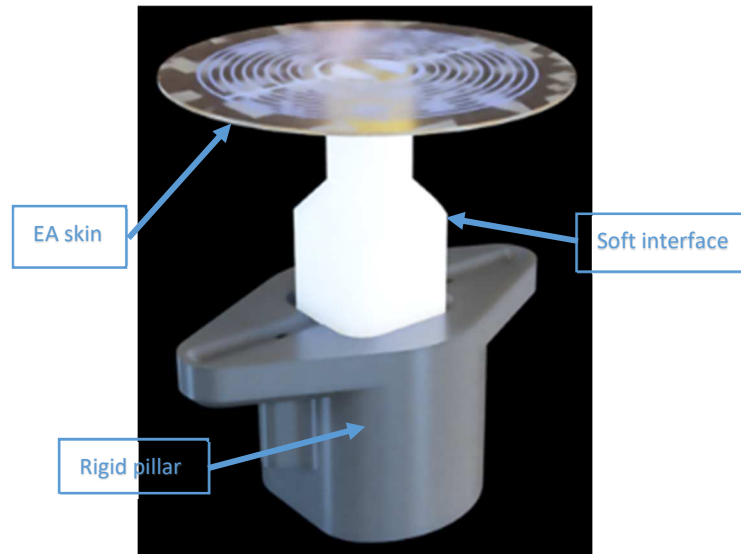
Figure 13. Rendering of the EA skin mounted on the rigid removable pillar through a soft pillar interface
